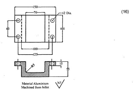
Prepare NC program in APT for machining the contour shown in Figure below with two passes one with rough-cut and other with finish cut.
